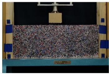
Figure 6: Arrangement of shallow foundation loading test equipment
