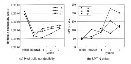
Figure 3. Variation of hydraulic conductivity and SPT-N value.
