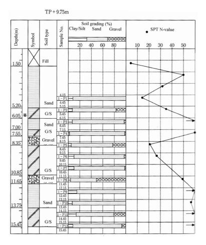
Figure 1. Soil profile, soil composition and SPT N-value of test field.
